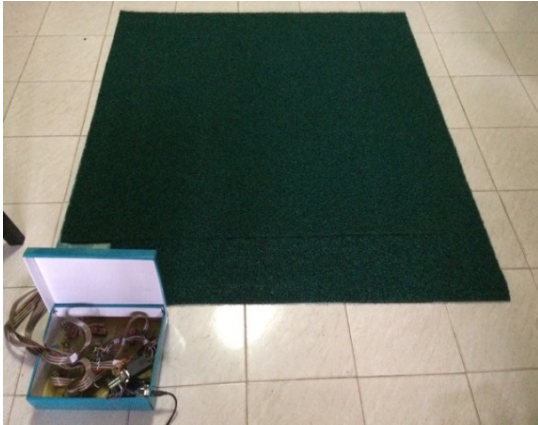
Fig. 3: The pressure sensitive mat is made of PVC fabric and is connected to a controller box to transmit signal to PC for analysis
