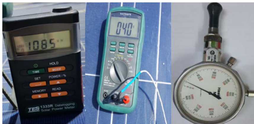
Fig. 14(a-c): Measurement devices, (a) Solar power meter, (b) Temperature sensor and (c) Tacho meter
