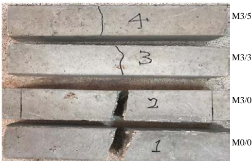
Fig. 6: Crushing of beams to find flexural strength for different mixes; M3/5, M3/3, M3/0 and M0/0
