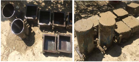
Fig. 2: Preparation of cylindrical and cubes
