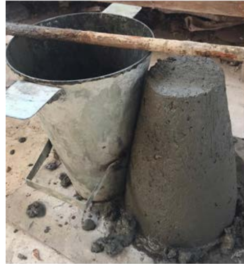
Fig. 4: Sample of Slump test for different mixes
