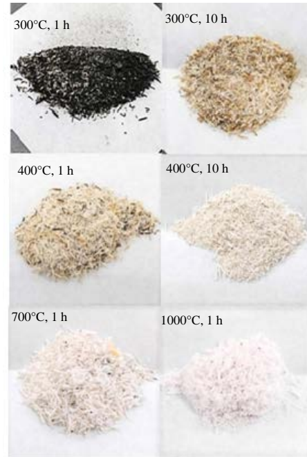
Fig. 2: The photograph of the overview of the RHA after firing at each temperature and time
