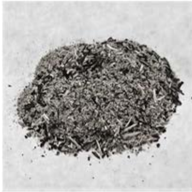
Fig. 1: The Photograph of the overview of the fired RH at 700°C for 1 h
