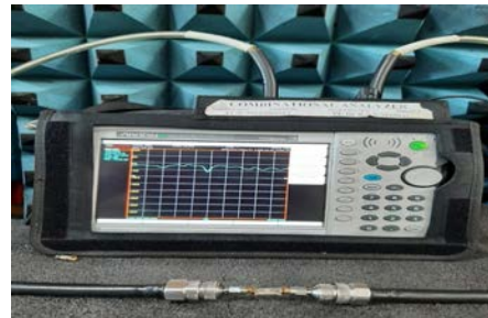
Fig. 3: Measuring the transmission co-efficient by using vector network analyser
