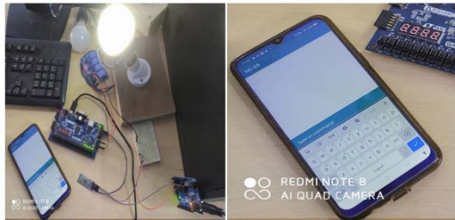
Fig. 13: Diagram for passing “1” from Arduino Bluetooth control app to the FPGA board
