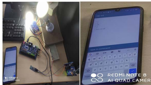
Fig. 17: Diagram for passing “turn on all” from the Arduino Bluetooth control app to the FPGA
