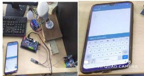
Fig. 16: Diagram for passing “9” from the Arduino Bluetooth control app to the FPGA
