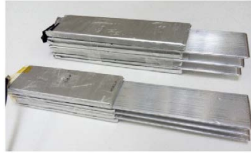
Fig. 3: The 8 Ah (top) and 3 Ah (bottom) battery packs with heat pipes
