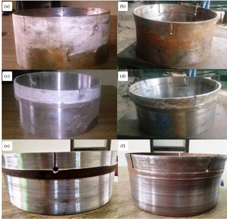
Fig. 6(a-f): Prototype samples of buffer casing (a, b) S2, (c, d) S3 and (e, f) S4 before and after application of 700 kN
