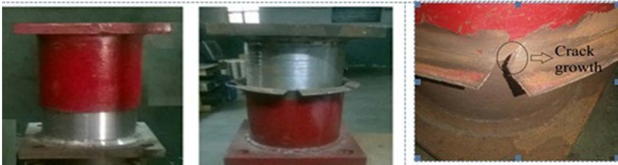
Fig. 5: Different views of S1 sample before and after testing showing generation of crack at 700 kN of load
