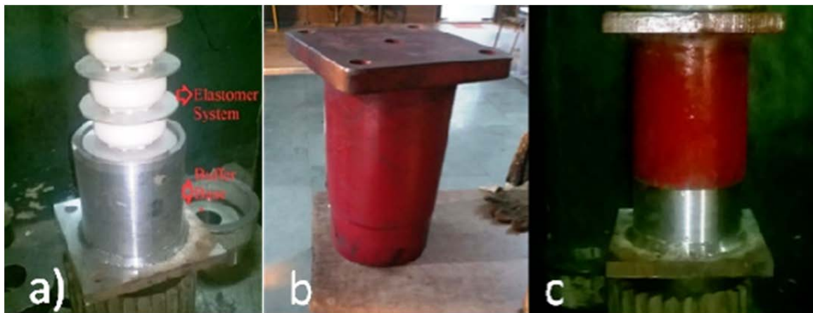
Fig. 1(a-c): Different stages of prototype crash (end) buffer fabrication
