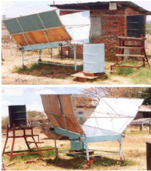
Fig.2: Photo of the prototype solar pasteurization system at Kenyatta University, Nairobi, Kenya
