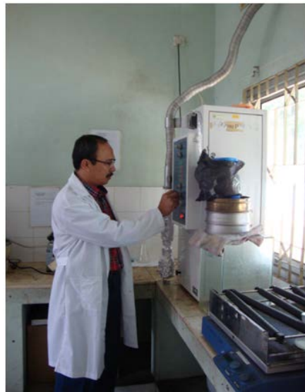
Fig. 1: Preparation of coating material for rice fortification by spray drying process
