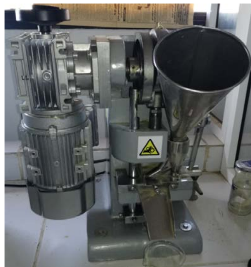
Fig. 4: Device for manufacturing tablets based on artichoke, bean and pea by-products
