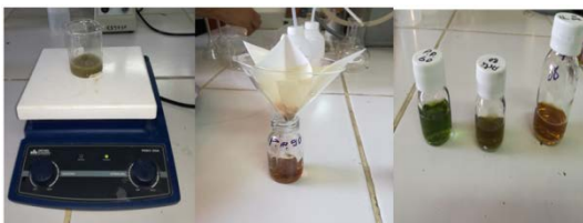
Fig. 3: Maceration with pure methanol and filtration
