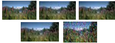
Fig. 7: Performance study of a communication system in Rician channels (SNR = 15dB) (a) Transmitted image (b) Received image in 2-PSK modulation techniques (c) Received image in QPSK and 4-QAM modulation techniques (d) Received image in 16-QAM modulation techniques
