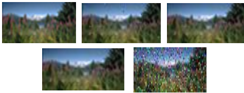
Fig. 3: Performance study of a communication system in AWGN channels (SNR = 15 dB) (a) Transmitted image (b) Received image in 2-PSK modulation techniques (c) Received image in QPSK and 4-QAM modulation techniques (d) Received image in 16-QAM modulation techniques
