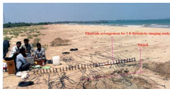
Fig. 2: Tsunamigenic deposits field work data collection using 2D ERI electrode arrangement and open trench technique
