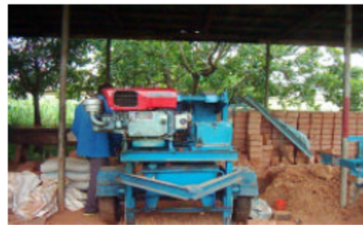
Fig. 2: Interlocking machine developed by NBRI, Ota. Source: Researcher's field survey (2005), Ondo State housing corporation, Akure
