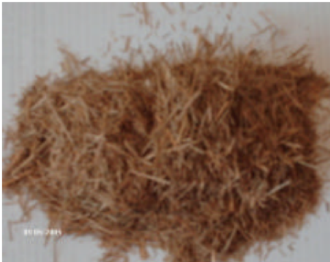
Fig. 4: Boiled crushed Diss fibres
