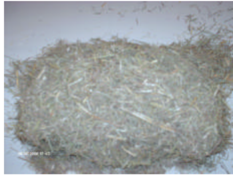
Fig. 3: Crushed natural Diss fibres
