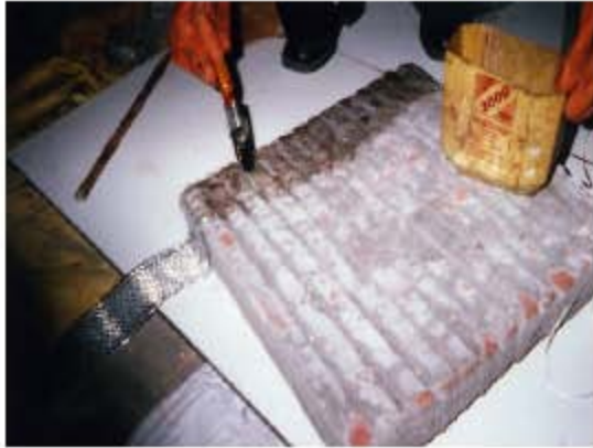
Fig. 8: Specimen treated with 2 strips
