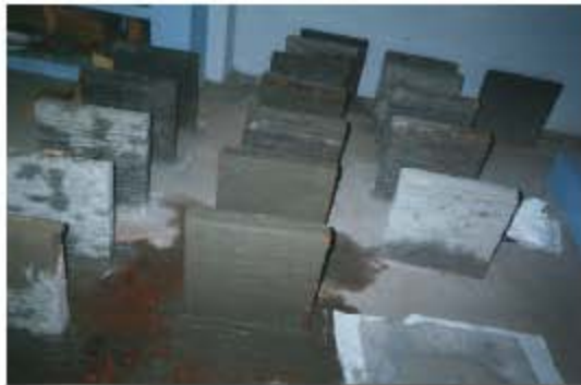
Fig. 4: General view of masonry wall panels under curing
