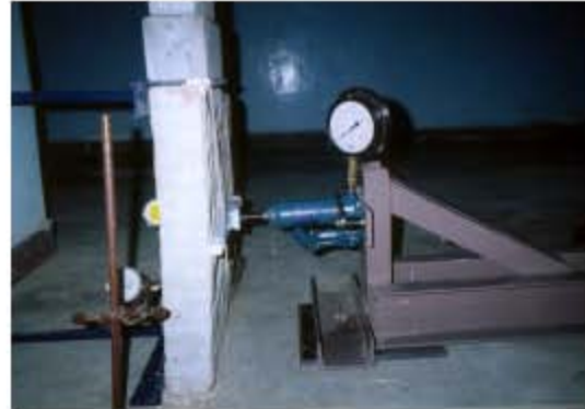
Fig. 5: Experimental set-up with pre-calibrated hydraulic jack
