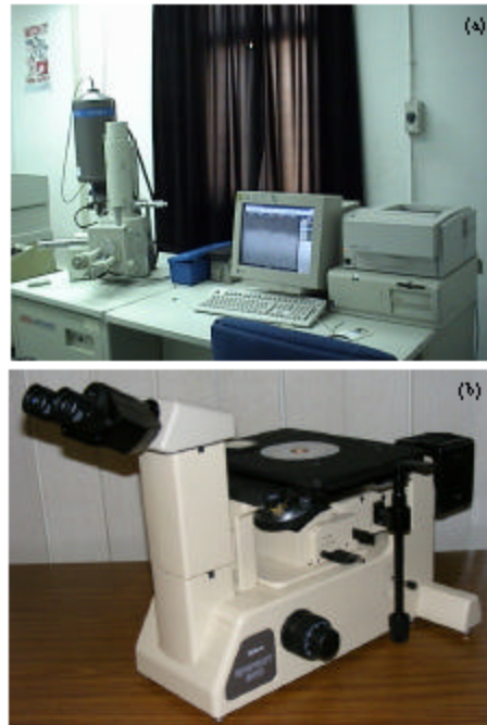
Fig. 1: a): Scanning Electron Microscope (SEM) and b): Optical microscope used for chip analysis
