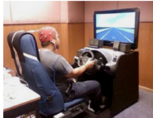
Fig 1: Driving simulator system
