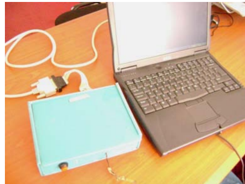
Fig. 3: Diagram of a Basal Body Temperature (BBT) logger interfaced with a personal computer
