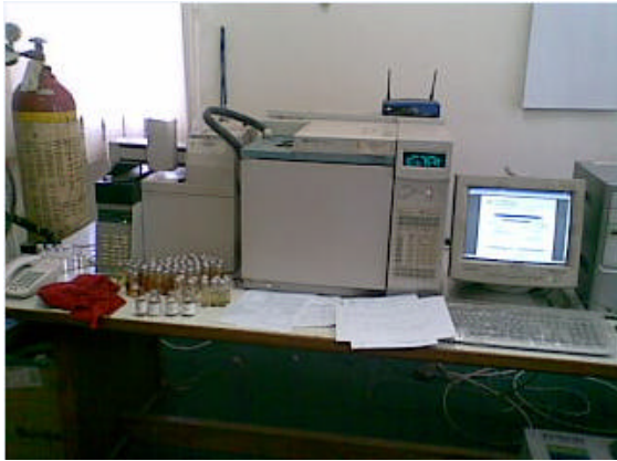
Fig. 4: Gas chromatograph for dissolved gas analysis
