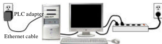
Fig. 5: Good separation with separate outlet for PLC wall adapter (Liu et al. , 2001)
