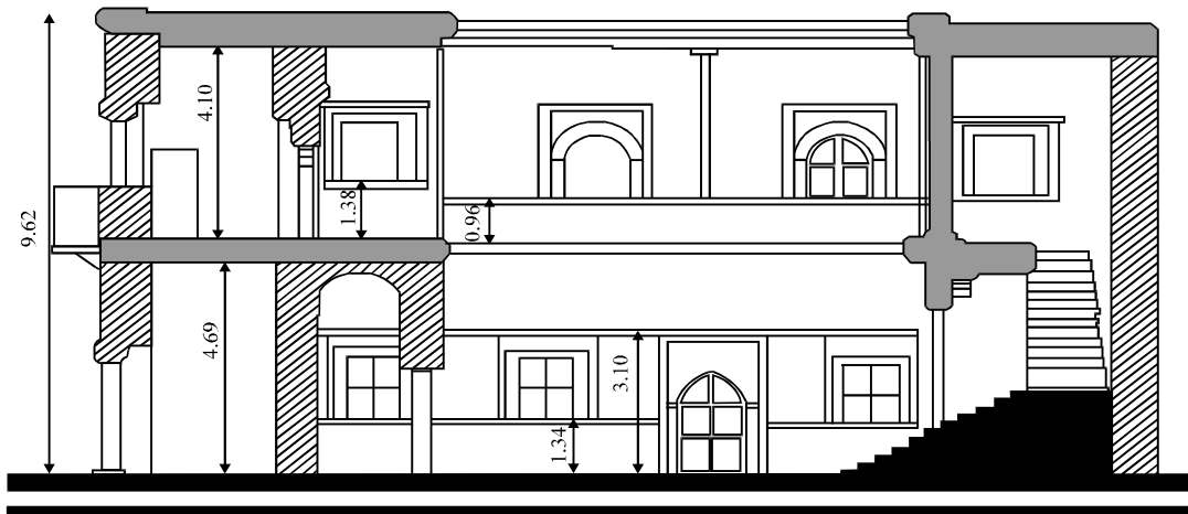
Fig. 8: Section through the house above
