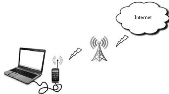
Fig. 2: Tethering using the smartphone as a modem
