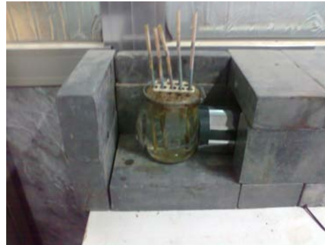
Fig. 1: Experimental arrangement for void fraction measuring equipment
