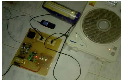
Fig. 6: LoWPAN node in source station sending TCS data to server
