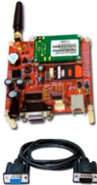
Fig. 9: SIM3000CZ microcontroller board with RS-232 cable
