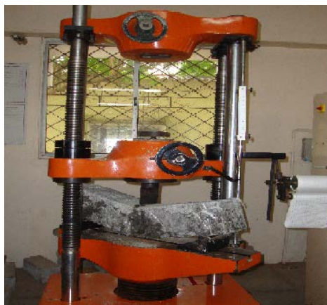
Fig. 7: Failure pattern of flexural strength of prism
