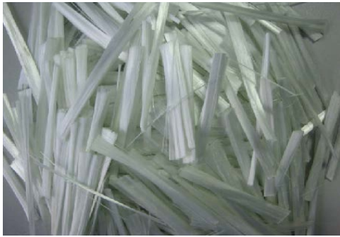
Fig. 1: Anti crack W70 AR glass fibre
