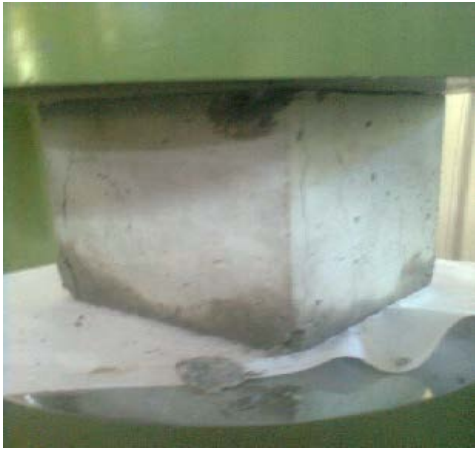
Fig. 5: Failure pattern of compression strength of cube
