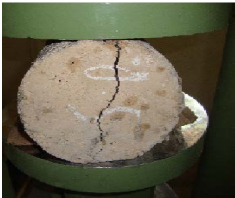
Fig. 6: Failure pattern of split tensile strength of cylinder
