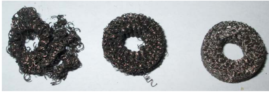
Fig. 2: Sleeves of different wire diameter after wearing; Left: d_w = 0.2 mm; middle: d_w = 0.15 mm and right: d_w = 0.1 mm
