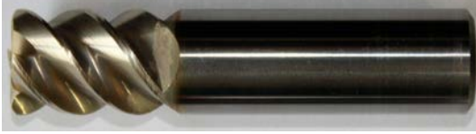
Fig. 1: Prototype end mill with normal tooth
