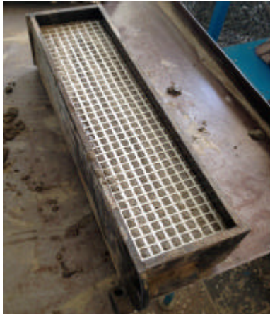
Fig. 8: The application of the second layer of mesh
