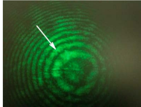
Fig. 4: Breaks on isochromes in the conoscopic picture of a monocrystal of paratellurite 40 mm thick received in the direction of an optical axis in a conic bunch of laser light with a wavelength of 533 nm. The arrow specified the largest break on isochrome of the 2nd order
