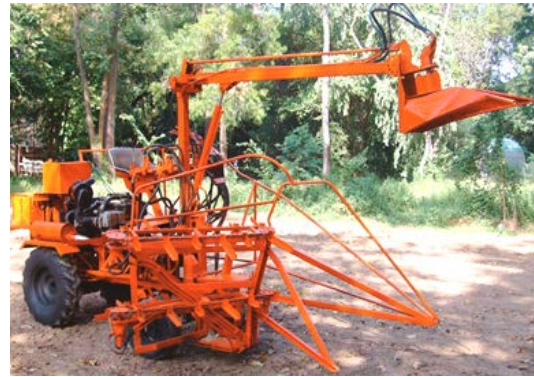
Fig. 1: Small sugarcane harvester
