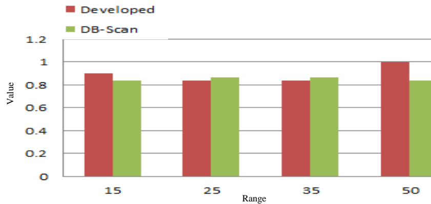
Fig. 11: Effects of different transmission ranges on the end-to-end delay values
