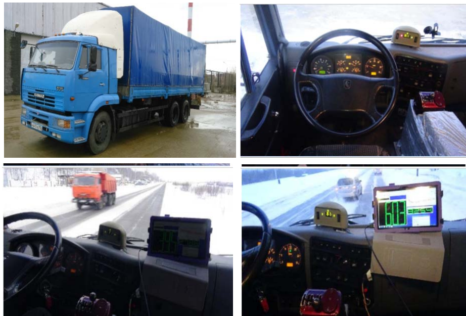
Fig. 5: Location of the display and the controller in the cab of KAMAZ 65117
