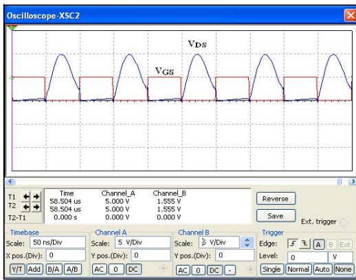
Fig. 7: a) binary signals an; b) the required Class-E power supply
