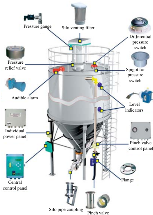
Fig. 2: Cement Silo safety system
