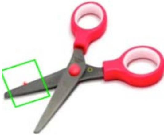
Fig. 12: Grasp point for open scissors; X_c = 33 , Y_c = 142 , Ang = 209 , t = 2.016619 sec
