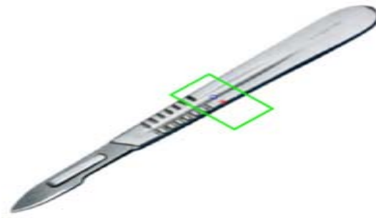
Fig. 17: Grasp point for a scalpel with a narrower gripper; X_c = 128 , Y_c = 105 , Ang = 459 , t = 2.119956 sec
