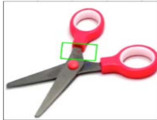
Fig. 13: Grasp point for open scissors with narrower gripper; X_c = 109 , Y_c = 96 , Ang = 852 , t = 1.850442 sec
