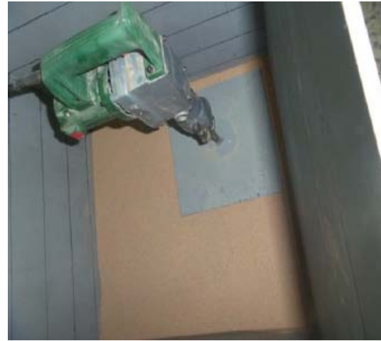
Fig. 6: Compacting soil model by modified jack hammer
