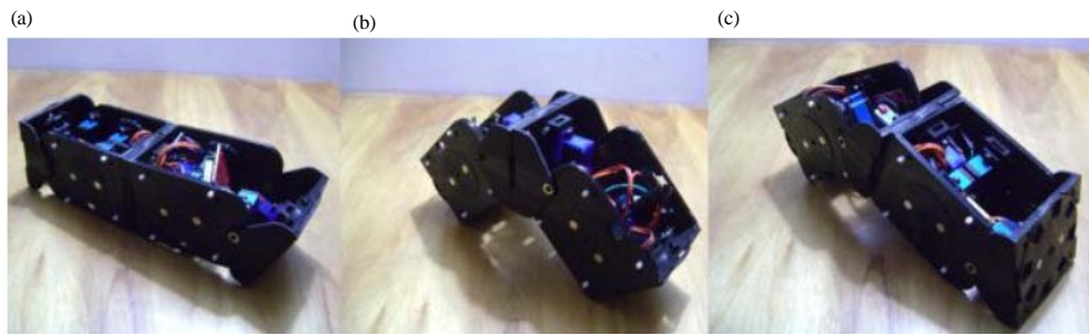
Fig. 3: Sub-module adjustments for MecaBot-3; a) Sub-configuration 1; b) Sub-configuration 2 and c) Sub-configuration 3
