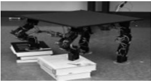
Fig. 2: Self-balancing table based on a quadruped's gait (Arredondo, 2006)
