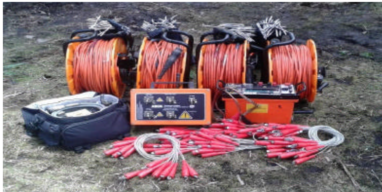
Fig. 8: ABEM SAS 4000 Terrameter with its accessories
