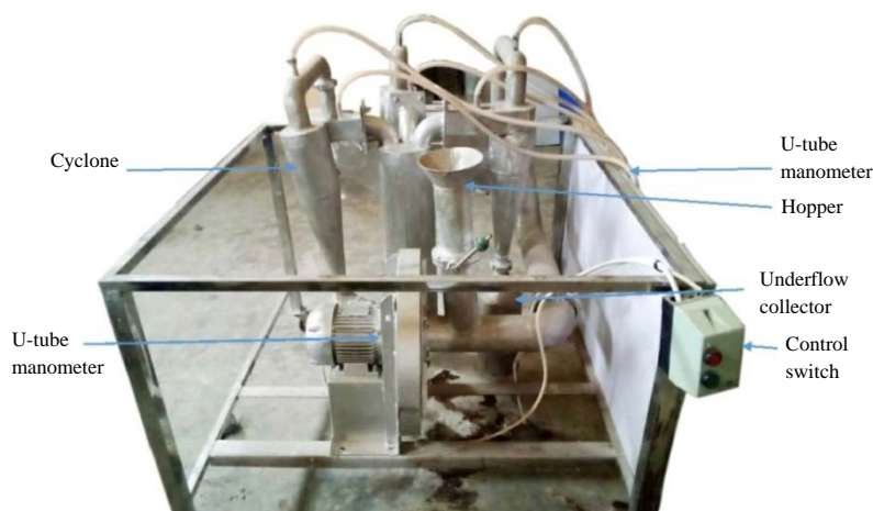
Fig. 2: A view of the designed and constructed parallel air cyclone rig for kaolin beneficiation
