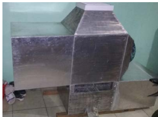
Fig. 4: Two levels indirect-direct evaporative cooler results
