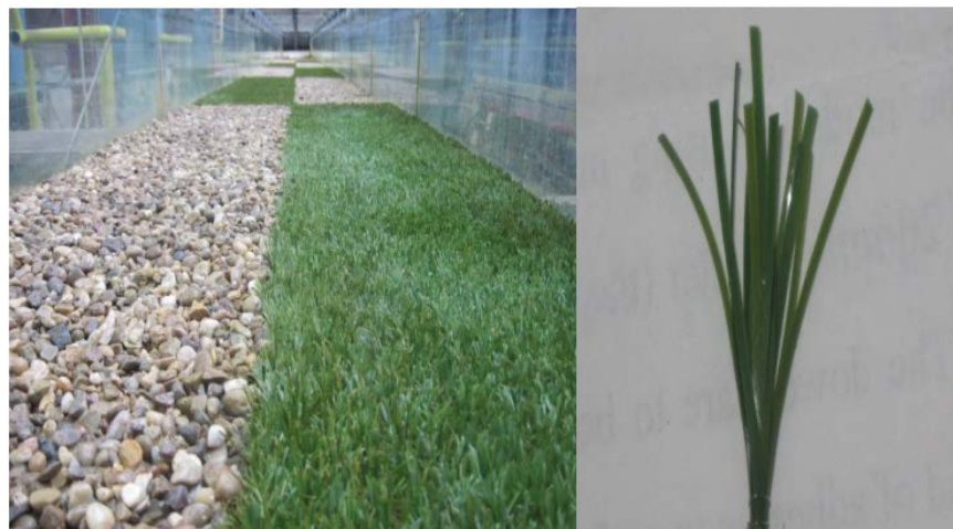
Fig. 2: Flume channel bed roughness variations and grass plant consisting 16 stems
