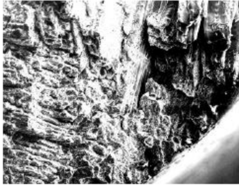
Fig. 5: SEM fracture surface of soldered Minalux specimen no. 2 ( N=1665250 cycle, \sigma = 250 MPa), X 125
