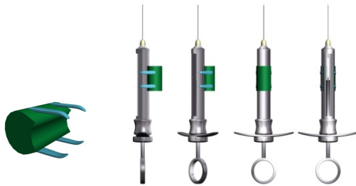
Fig. 1: Dental Injection Pain Reducer Instrument (DIPRI) scheme (left) and its schematic attachment position of on dental injection syringe (right)
