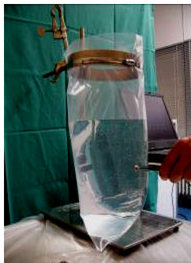
Fig. 1: Set arrangement of soft tissue simulator and microphone
