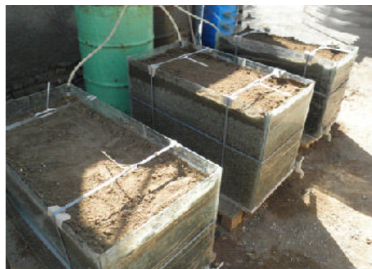
Fig. 1: Glass pilot plant of subsurface flow wetland
