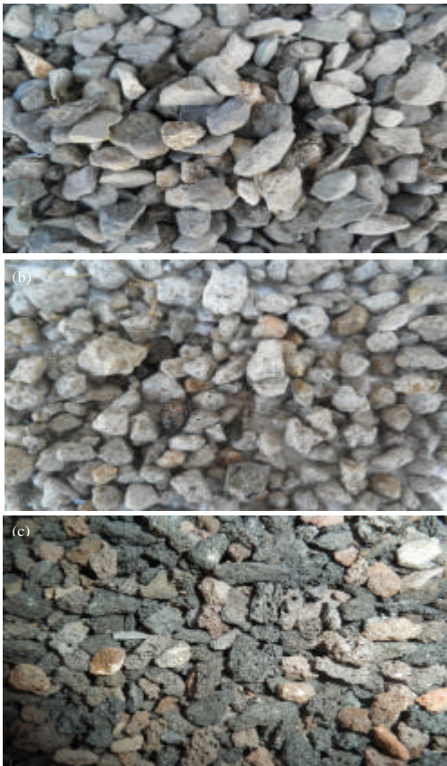
Fig. 2: The filling material of the bed: a) sand; b) escoria stone and c) pamis stone
