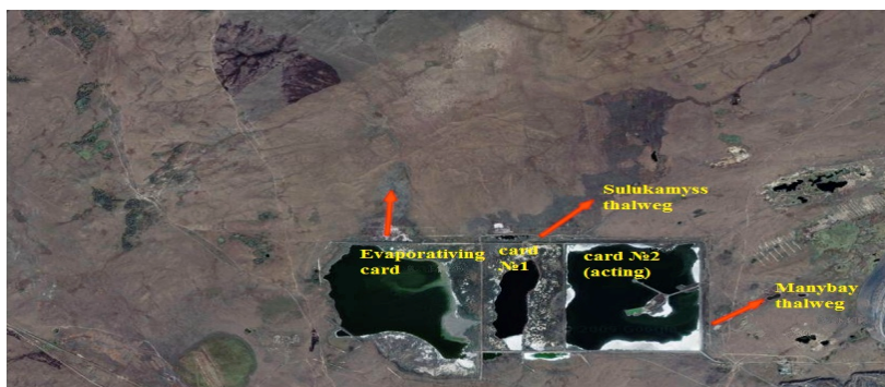
Fig. 1: Space photo tailings HMP (red arrows indicate the spreading of groundwater from the tailings cards)
