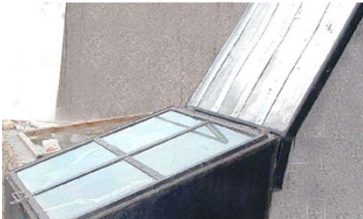
Fig. 3: Experienced helio-camera for heat treatment of concrete two-way supply of thermal energy Kyzyl-Orda
